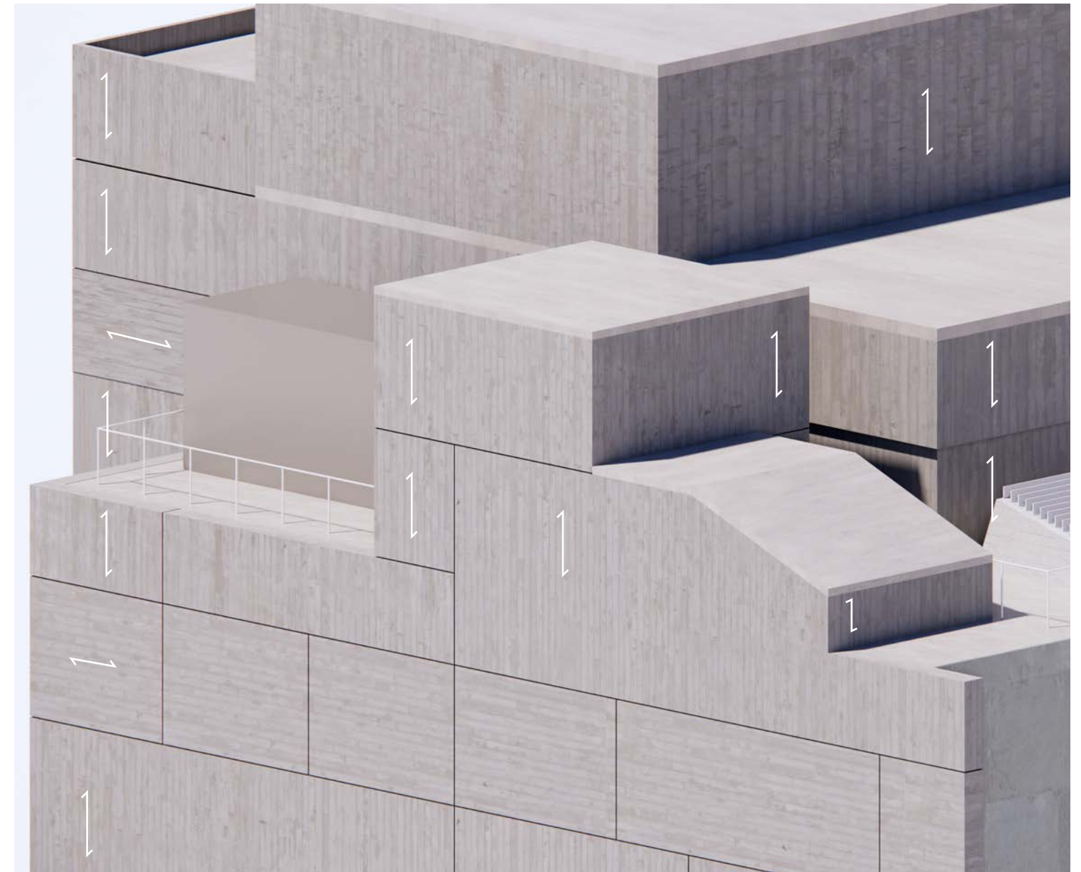
Addition of elevator bulkhead with board-formed concrete to match existing as much as possible. Formwork orientation to be vertical - same as all typical rooftop walls Introduce horizontal control joint aligned with top of existing stair bulkhead wall
