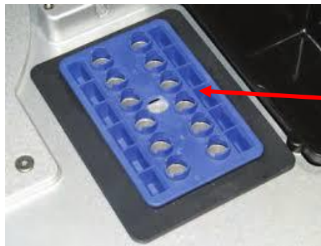
sample plugs placed in these slots
