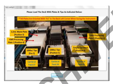
3.12.9 Add another Promega 2.2ml deep well plate under position 4 on carrier on tracks 41-47. The plate should rest on top of two Nunc plates (used for elevation only) as seen in the photo below.
