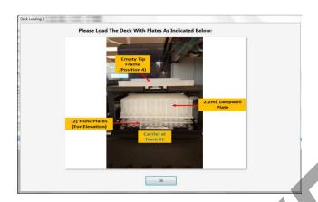
3.11.10 Refill tips as needed according to photo below. Ensure that correct size tips go in correct carrier. Ensure that the bar code on the side of the tip tray is facing to the right.
