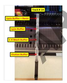
3.10 Load the indicated volume of each reagent into new 60ml reagent containers on track #14 as indicated by the arrows above. The calculation of the amount of reagents is calculated by the robot software. The following tables may also be used for reference.
