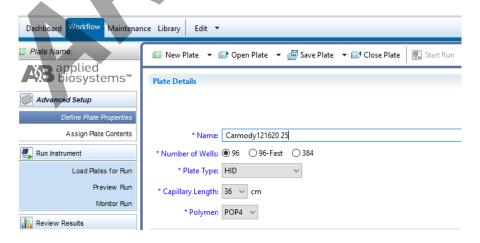
2.21.1 Name your plate using the naming system based on the instrument, date, and injection number(s) (i.e. Carmody121620 25).
