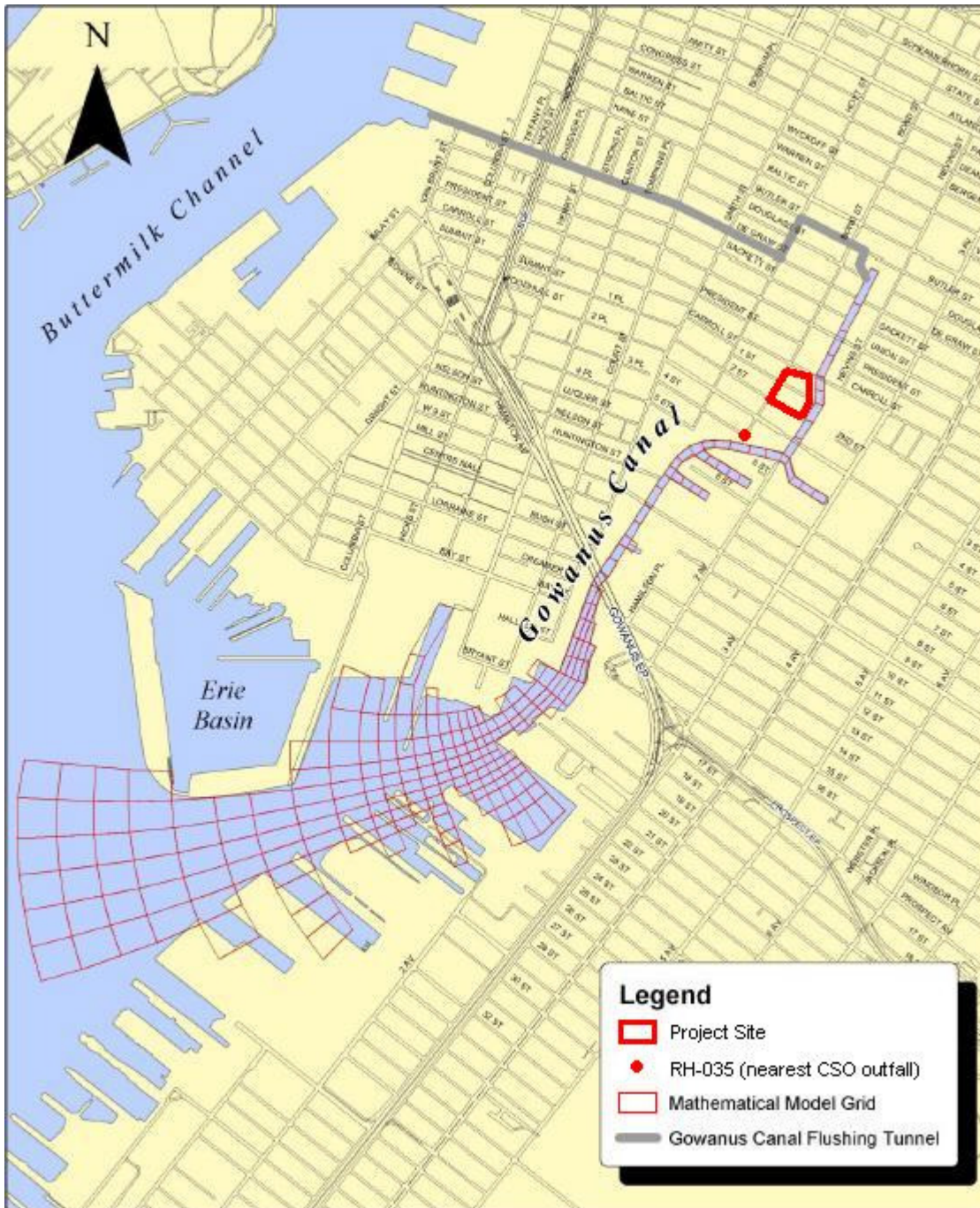
Figure 6. Water-Quality Model Grid
