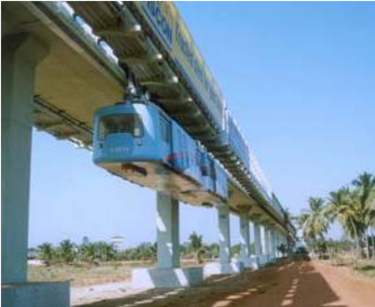
The SkyBus on the Goa test track. Similar to the JFK Airtrain in New York, SkyBus technology increases the amount of people who can use a transportation right-of-way without increasing congestion. Image used with permission of SkyBus-Atrilab.
