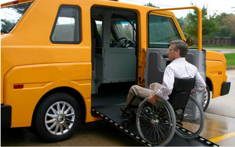
The Standard Taxi features a lowered chassis and a built-in wheelchair ramp. It holds four passengers in addition to a wheelchair. Image used with permission of The Vehicle Production Group LLC ( www.standardtaxi.com ).
