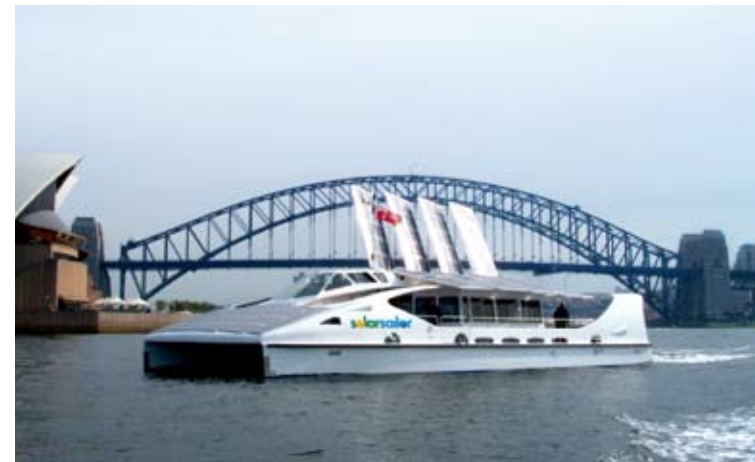
The original Solar Sailor in Sydney harbor operated by Captain Cook Cruises. The wing panels serve as sails while simultaneously collecting solar energy. Image used with permission of Solar Sailor ( www.solarsailor.com ).
