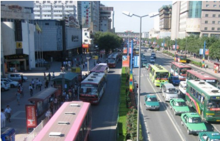
A physically separated, designated right-of-way for buses in Xian, China. NYC Dept. City Planning
