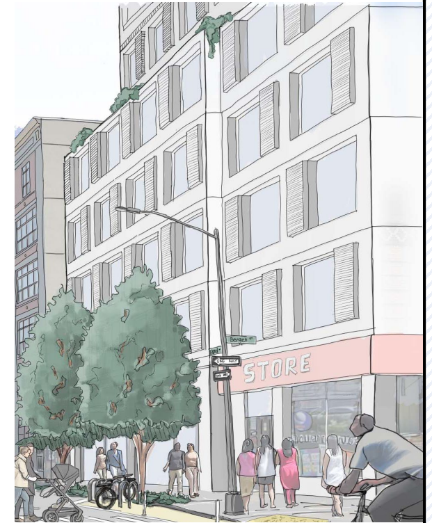
Example sketch of required street wall recess
