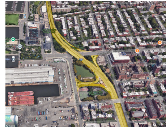
Curves and Limited Stopping Sight Distance from Congress Street to Joralemon Street
