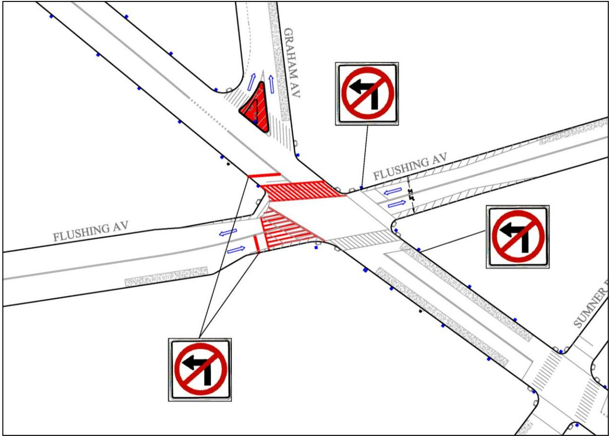
*Figure 53: Proposed Crosswalks and Concrete Islands at Broadway and Flushing Avenue*
