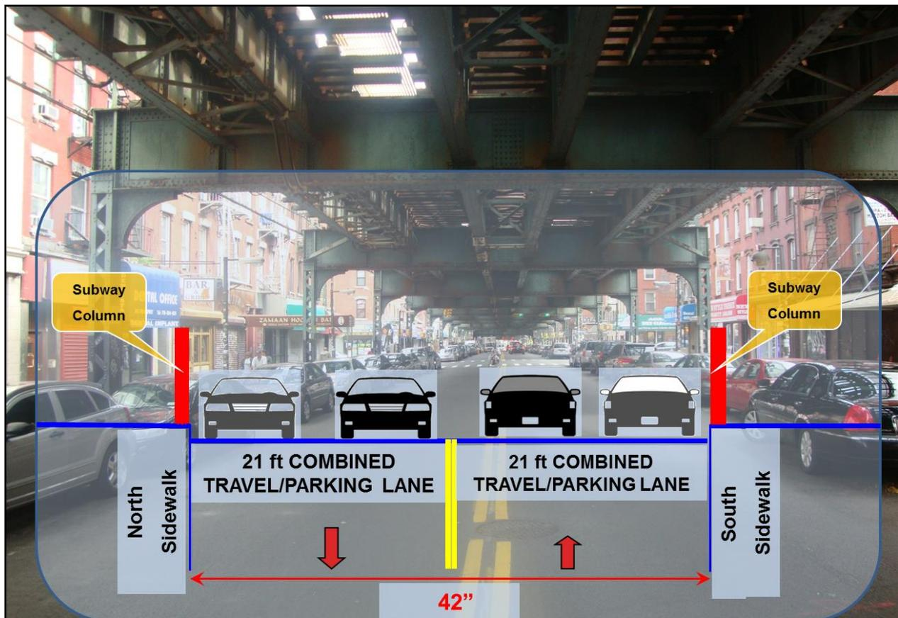
*Figure 3: Broadway Typical Cross Section*
