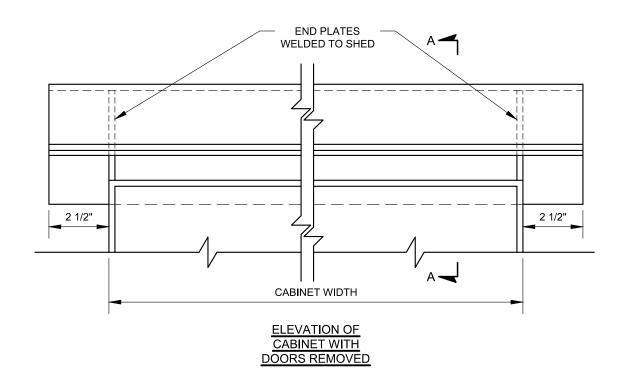
MATERIAL: 1/4" BOILER PLATE STEEL
