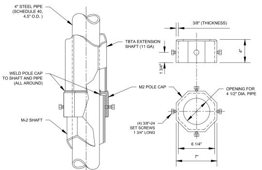
M2 POLE CAP DETAIL (CAST STEEL)
