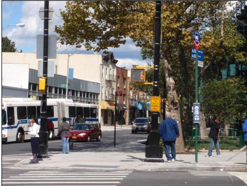
*Figure 15: Pedestrian Countdown Signals along the White Plains Road Study Corridor*
