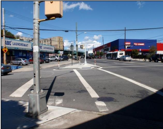
*Figure 28: Recently installed raised island between the southbound right turn bay and the southbound approach at the White Plains Road and Sagamore Street intersection*
