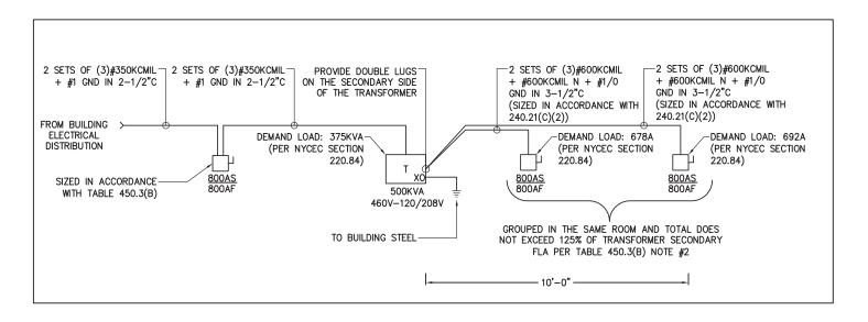
1. THE LENGTH OF THE TRANSFORMER SECONDARY CONDUCTORS, AS DENOTED IN THE DRAWING, SHALL NOT EXCEED 10 FEET.
