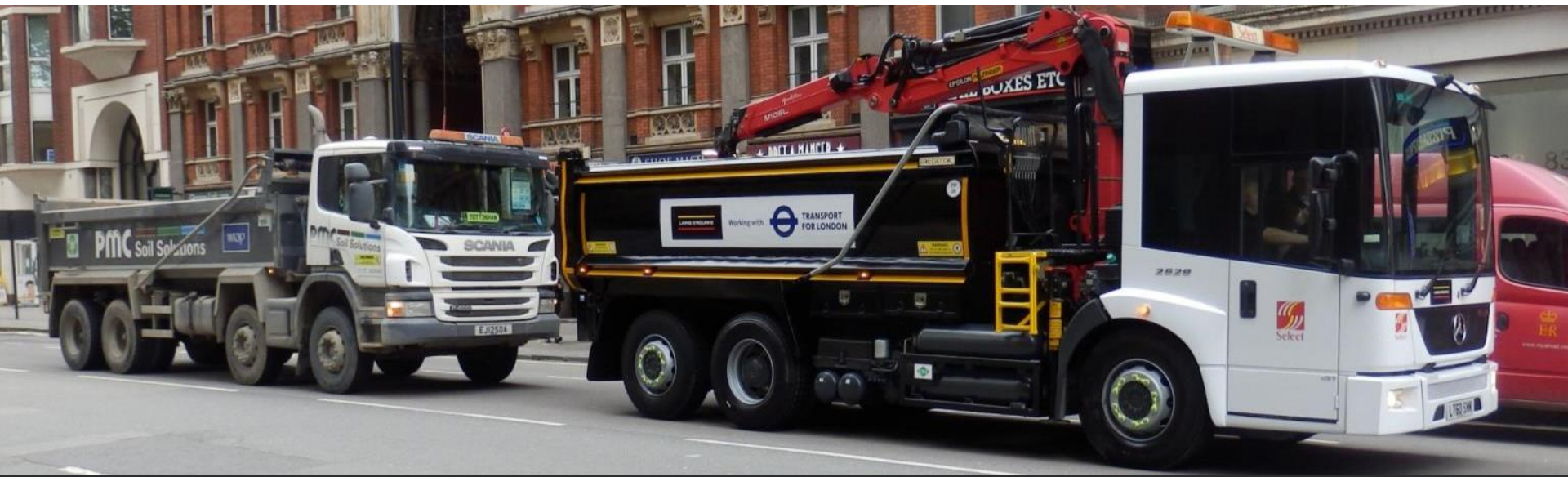
Utilisation of cabs with 'best-in-class' driver direct vision
