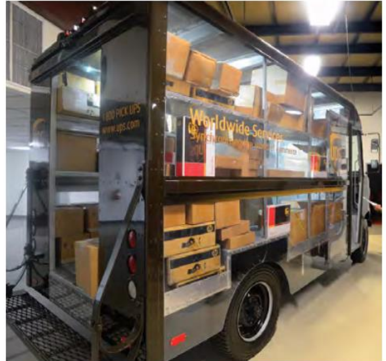
▶ See through package delivery vehicle allows trainers to ensure trainees learn safe loading techniques, Landover, Maryland, U.S.
