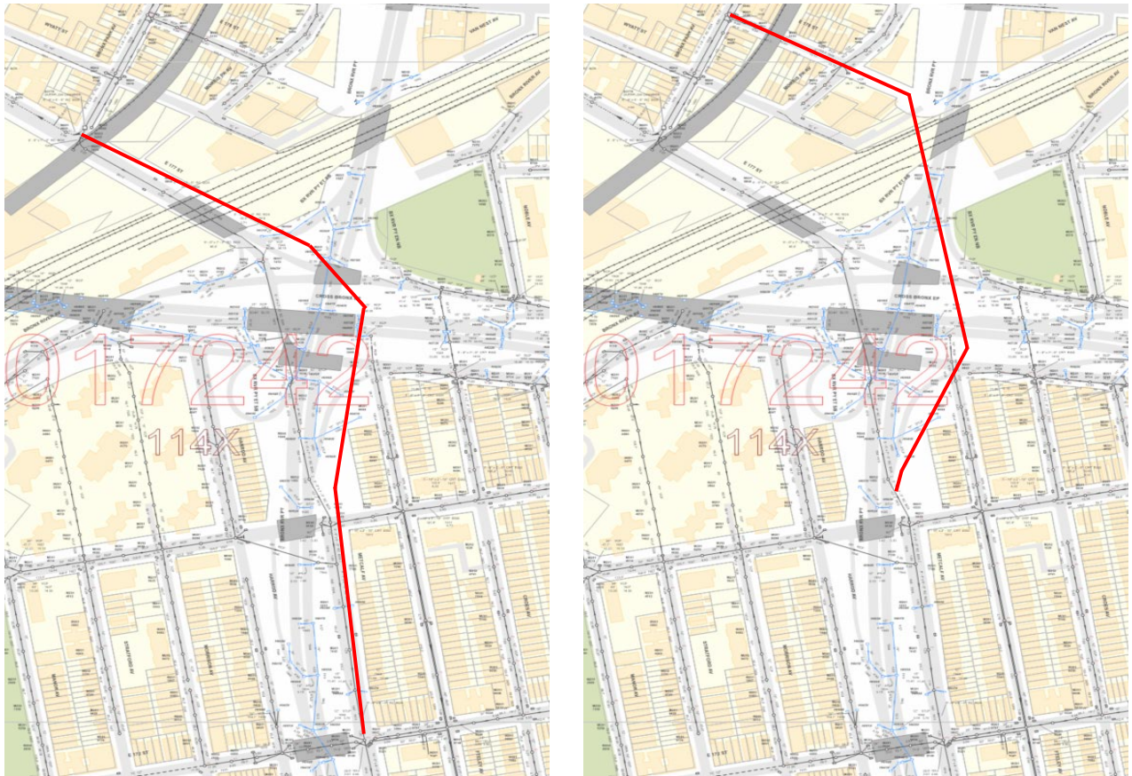
Figure 2 Comparison of relief sewer configuration in LTCP (left) and BODR (right) at HP-007
