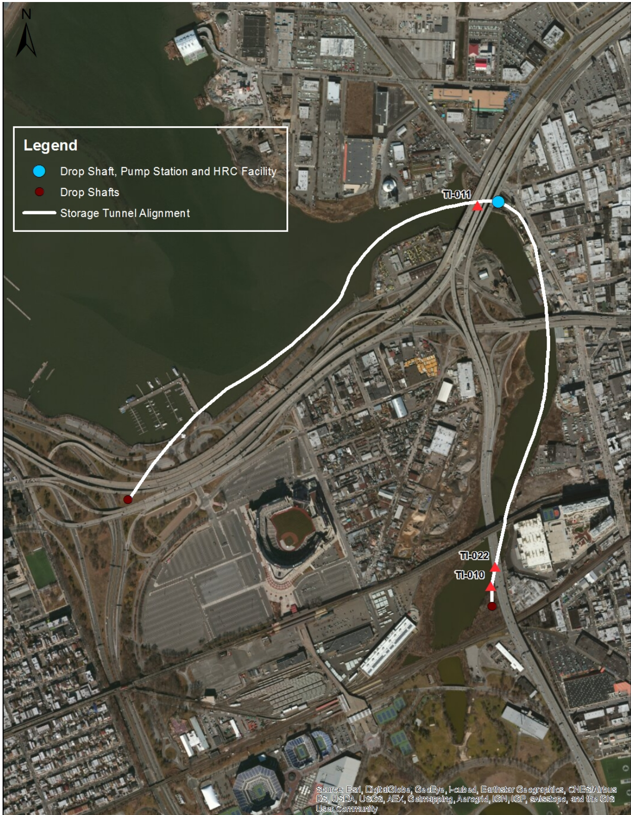
Figure 8-4. Proposed Route of 100 Percent CSO Volume Tunnel
