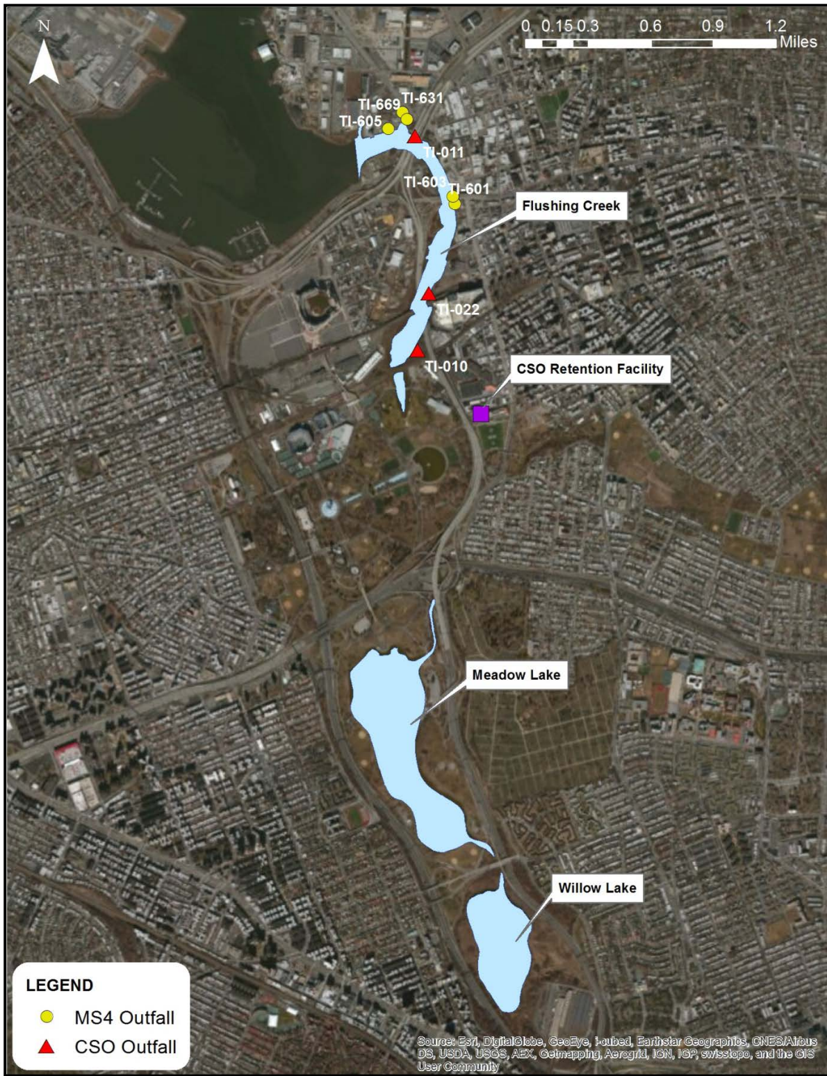
Figure 2-7. Flushing Creek SPDES Permitted Outfalls
