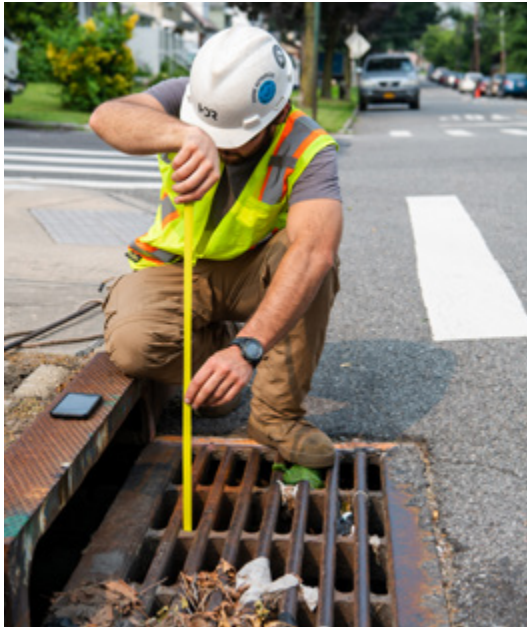
Measuring debris in catch basin for Loading Rate Study
