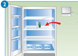
Use a continuous digital data logger with a buffered probe as both the primary and backup thermometer.
