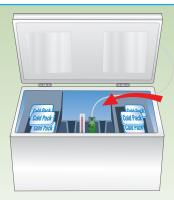
In a chest freezer, place the probe of the continuous digital data logger next to the vaccines.
