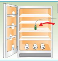
Place the probe of the continuous digital data logger in the center of the refrigerator.
