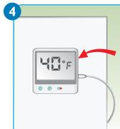
Attach the display of the continuous digital data logger to the outside of the refrigerator, either on the door or on the side. Set the temperature range.
