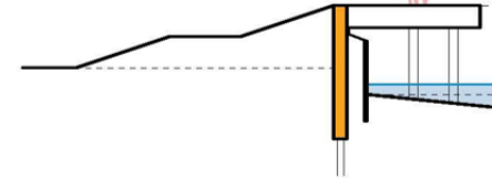
Bulkhead (or Caisson)
