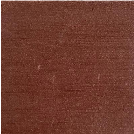
Pigmented Architectural Concrete
