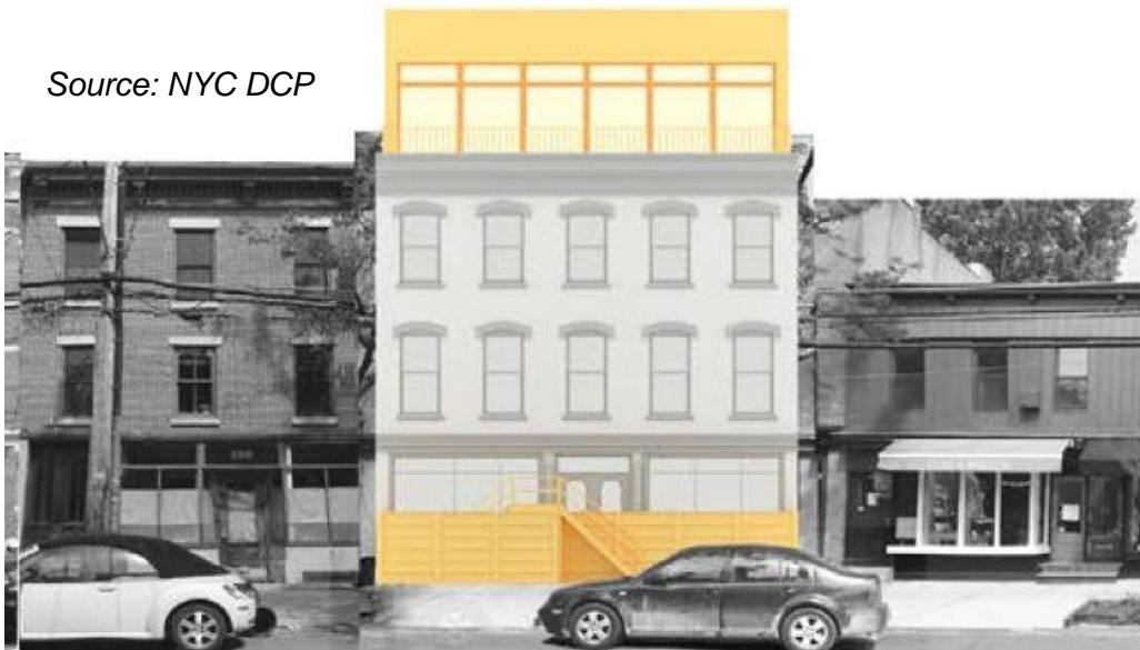
Building-level approaches may involve a combination of floodproofing and relocating critical systems, possibly abandoning the basement
