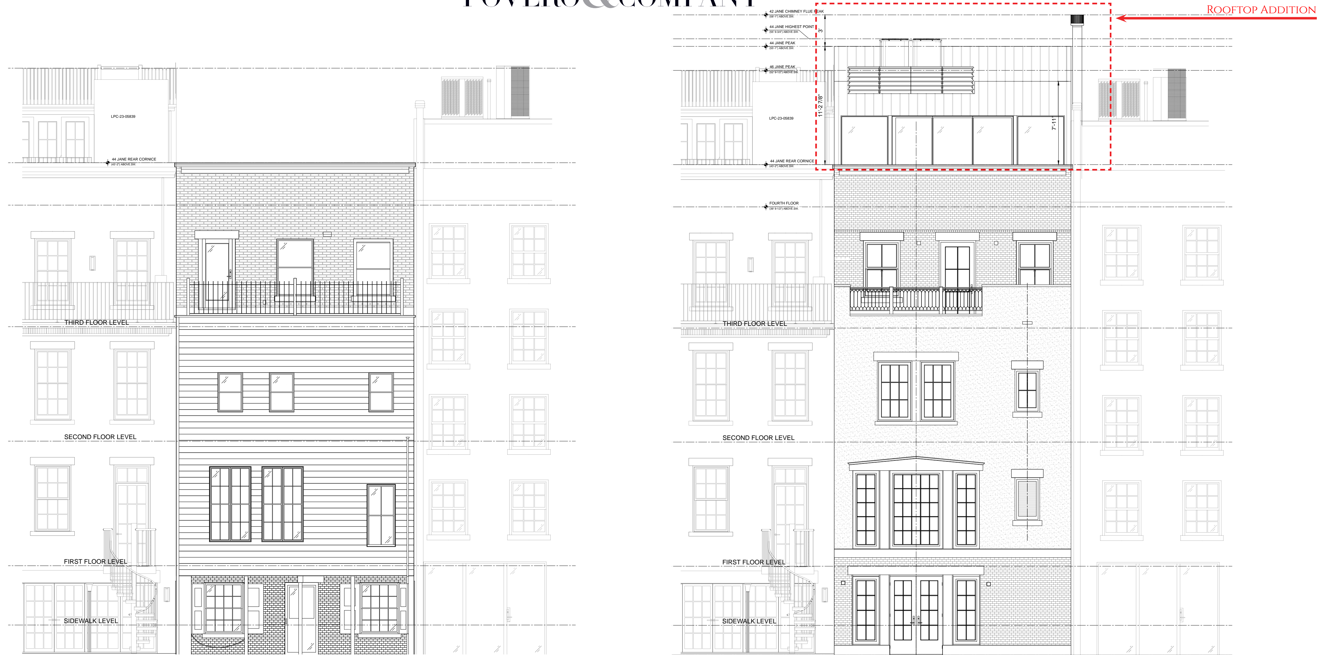
EXISTING & PROPOSED REAR ELEVATIONS
