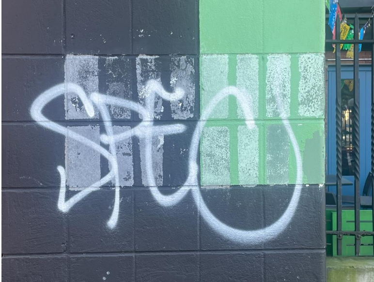
Test area tagged between first and second applications of the removers.
