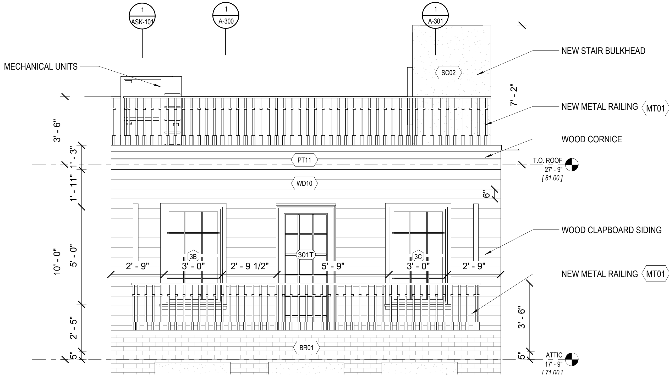
Top Floor Facade Elevation
