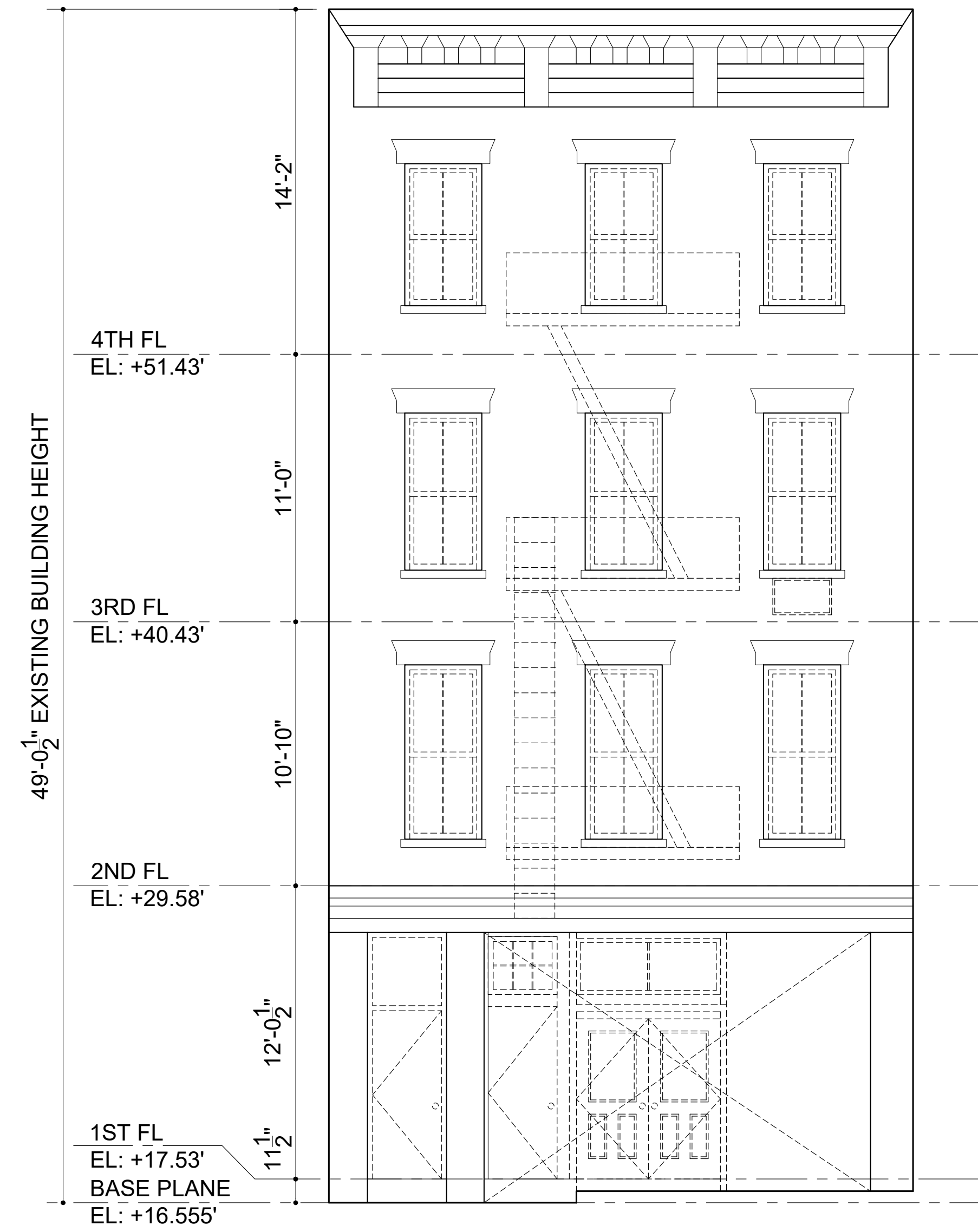
EXISTING GREENWICH ST ELEVATION
