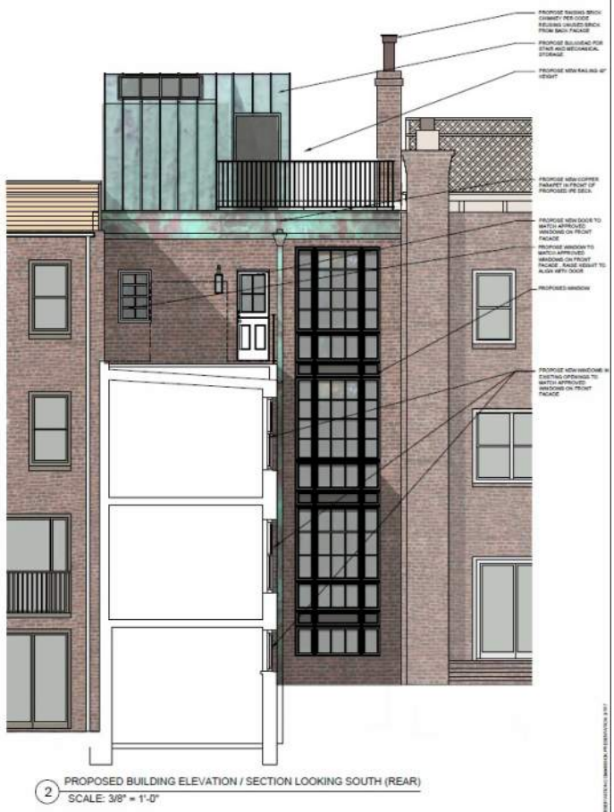
Rear facades of 75 and 77 Jane Street, rear additions and top floor rear façade reconstructions approved in 2015 and 2017, respectively.
