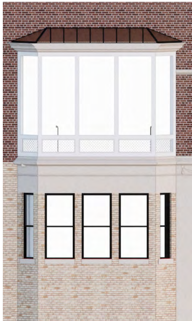
B1 SECTION DETAIL - WEST WINDOW BAY 1ST FLOOR CORNICE SCALE: 3" = 1'-0"
