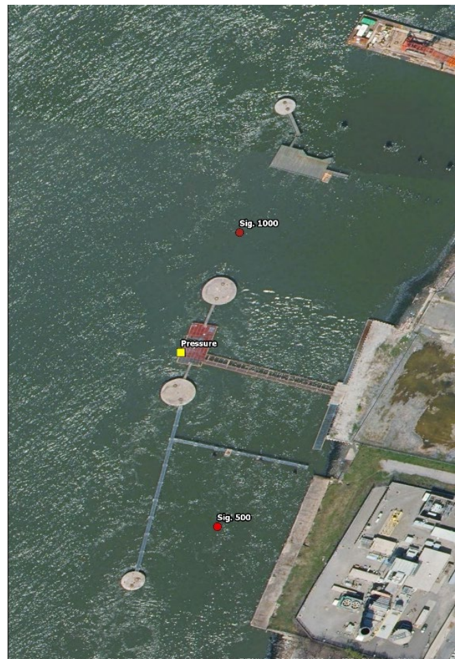
Figure 2-1: N1 st Street data acquisition deployment plan
