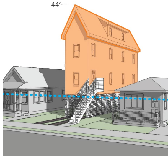
Existing Rules: maximum height of 35' as measured from the DFE or 9' Reference Plane
