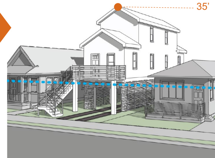
Proposed Rules: maximum height of 25' as measured from the DFE up to 10' Reference Plane
