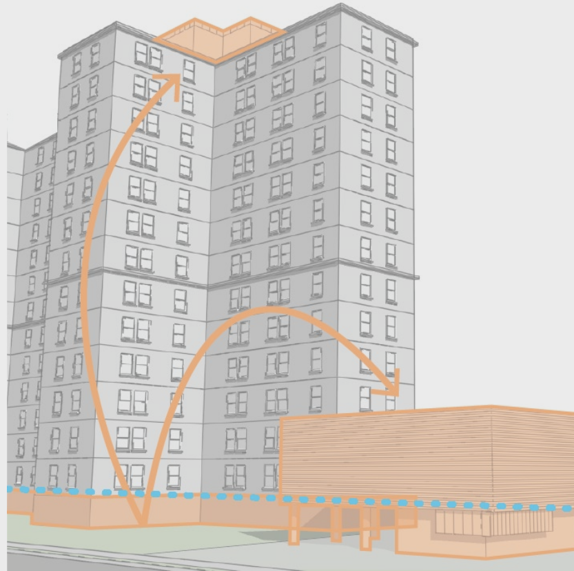
Proposed Rules: Additional flexibility to facilitate mechanical, electrical and plumbing equipment to be placed on the roof or in a separate structure
