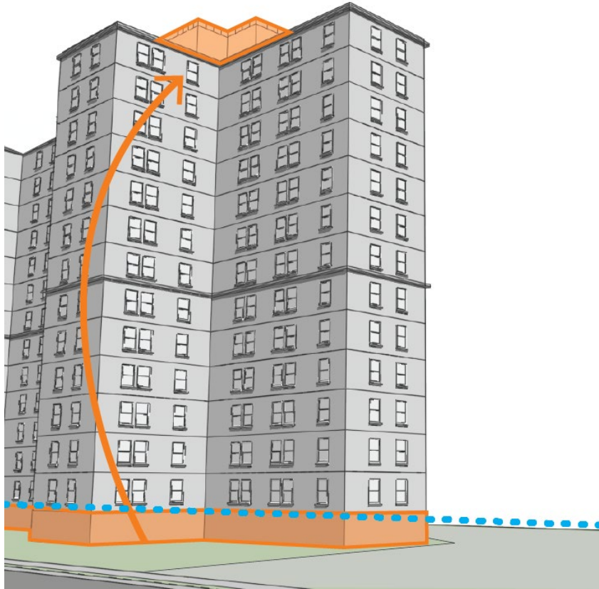
Existing Rules: Additional flexibility with permitted obstructions facilitate mechanical equipment to be relocated to the roof of buildings
