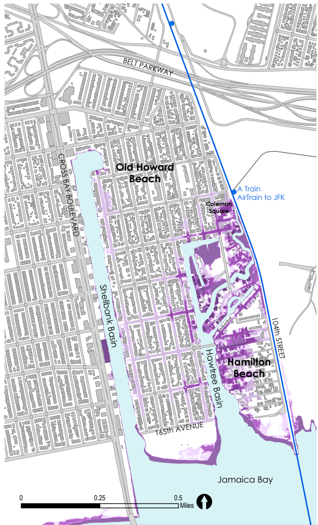
Extent of future daily tidal flooding based on sea level rise projections for 2050
